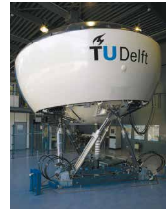
Simona Research Simulator was specially built for TU Delft and can realistically simulate all types of aircraft, helicopters and even cars.
